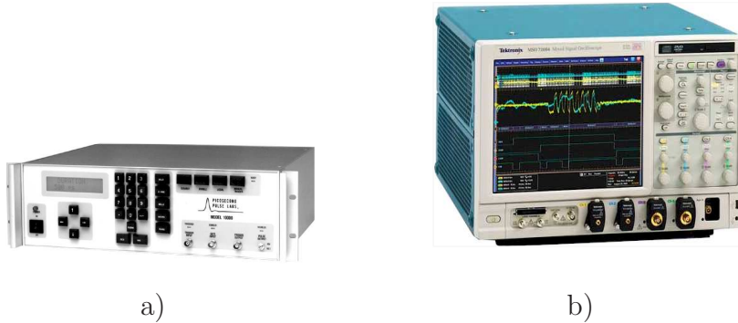
Figure 2. a) Picosecond Pulse Generator 10070A and b) Tektronix DSA70000 Series Real Time Oscilloscope
