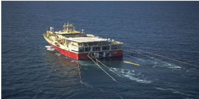
An array of 8 streamers, 6km long, pulled by a tugboat
