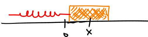
If  $k = 2 \frac{N}{m}$ , what is the work done by the spring on the block as it moves from  $x=0$  to  $x=.03$  m?
